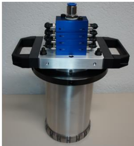
Diameter 140H6, 2x8 air jets : Measurement of roundness for truck engine bloc
